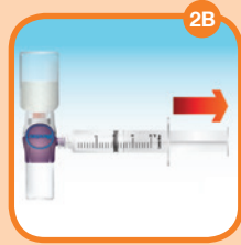
2B: With water vial at the bottom, attach syringe and pull plunger back to withdraw air
